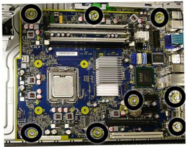
**11.** Lift up the front of the system board, and then pull the system board forward, up, and out of the chassis.
